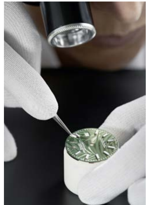
Setting up the appliques on the palm motif dial of the Oyster Perpetual Datejust 36
