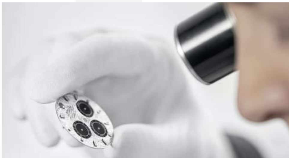
Quality control of the dial of the Oyster Perpetual Cosmograph Daytona
